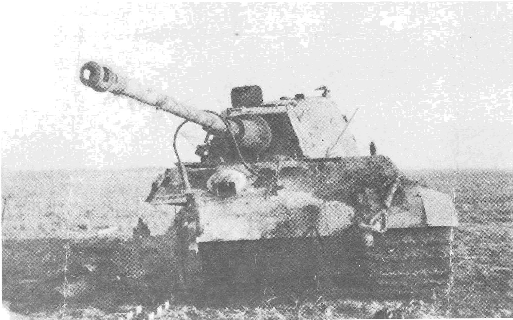
FIGURE 15 Tank knocked out by 823rd TD Battalion (equipped with 3-inch towed guns) shows ineffectiveness of hits on front glacis plate of Tiger II. At a range of 500 yards, frontal hits merely gouged out armor and ricocheted off. A track hit only partially severed the track, which did break completely as the tank attempted to back up.
